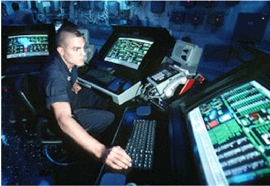
GSM2 Shane K. Hightower, a Ft. Pierce, Fla., native, monitors the damage control reporting system aboard USS Yorktown. This computerized system collects data on the status of the ship and feeds it through the local area network to five control stations, eliminating the need for messengers and phone talkers at various damage control stations. Should one control station be disabled, the others can still manage any battle damage problem.
